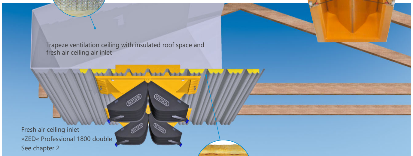
GRP / aluminium trapeze ceiling (approx. 3 mm wide slots), with fleece and 2-layer mineral wool
