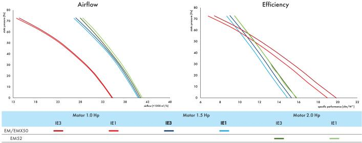
Airflow and efficiency data measured at standard conditions (20°; 1013 hPa). \*1 cfm/W = 1.7 m $^3$ /hW
